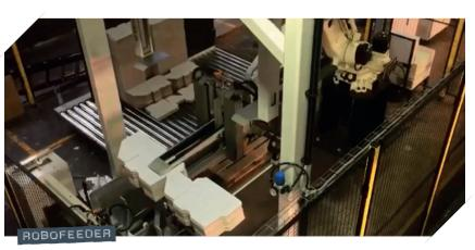
The flexibility of the robot allows the packages to be turned in all kinds of palletising patterns with a bottom sheet for pallet protection and an intermediate sheet between layers, up to a speed of 900 packs/hour. For palletising after inliners, the Robot Palletiser P3-3 includes a pre-stacker which increases the speed up to 1.400 packs/hour.
